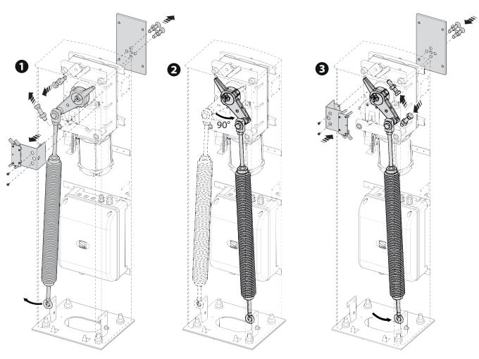
Install the boom-attachment cover on the anchoring plate with one screw only. Leave the screw slightly loose to make it easier to fit the boom later.
