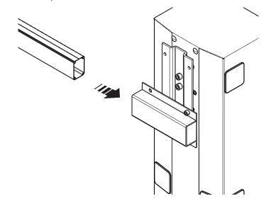
Position the boom vertically and fix it in place using the remaining screws.
