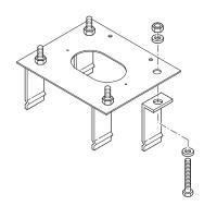
Fit the anchoring plate in the iron cage.
