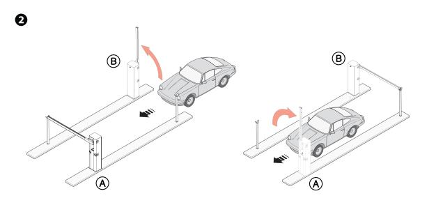
3 STEP-BY-STEP command (2-7) on barrier A or B for emergency opening
